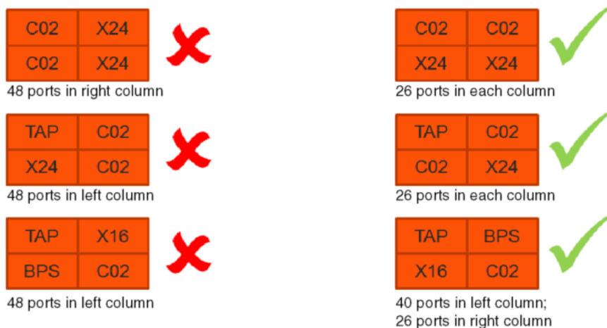
Figure 7 Module Placement of PRT-HC0-CO2, 100G Mode
